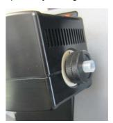
Fig. 9 - 26 Flow-through system ready for hose connection, front and back side
