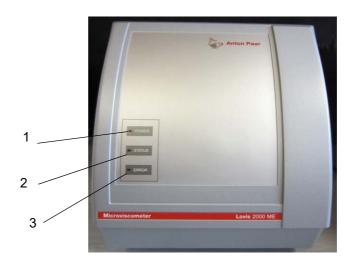
Fig. 5 - 4 Module Housing Lovis ME front view
