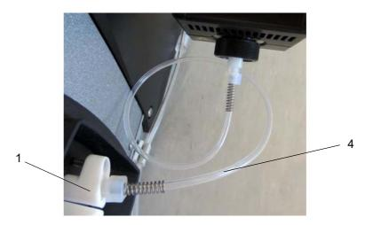
Fig. 22 - 5 Connecting the hose between DMA M and Lovis
