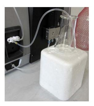
Fig. 19 - 5 Lovis + DMA M + Xsample 52: elevated sample vessel
