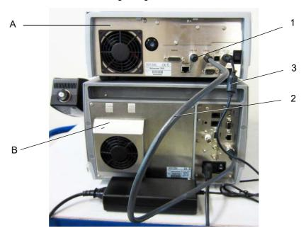
Fig. 22 - 3 Lovis 2000 ME + DMA M + Abbemat - connecting the cables
