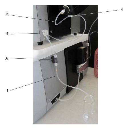
Fig. 18 - 4 Lovis + Xsample 52: Connecting the sample filling hose
