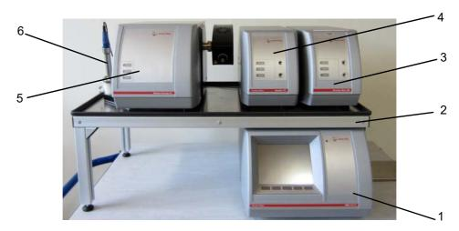
Fig. 20 - 12 Placing master instrument and modules - horizontal setup
