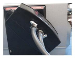
Fig. 6 - 8 Standard cooling hoses and hose clamps on Lovis capillary block
