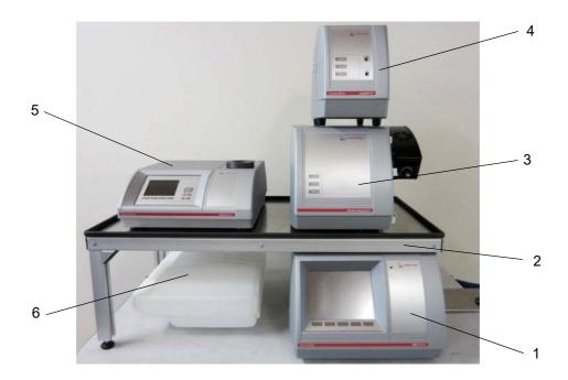
Fig. 22 - 10 Lovis 2000 ME + DMA M + HazeQC ME + Abbemat + Xsample 122/ 520 - Placing master instruments and modules
