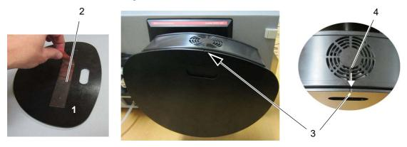
Fig. 17 - 5 Mounting the PVC crush protection
