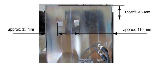
Fig. 19 - 7 Mounting the cable clips
