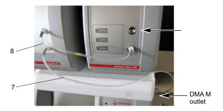
Fig. 20 - 7 Hoses master instrument outlet to Alcolyzer ME
