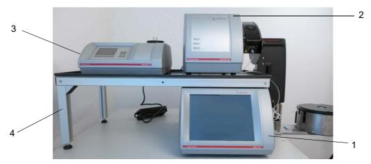
Fig. 22 - 27 Lovis 2000 ME + DMA M + Abbemat + Xsample 530 - Placing master instrument and modules
