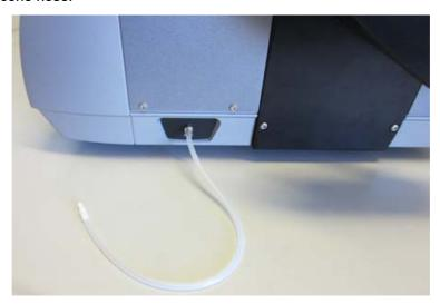
Fig. 6 - 1 Lovis 2000 M with air hose plus Luer cone connected
