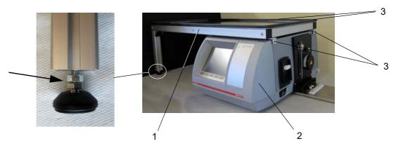
Fig. 20 - 11 Positioning the stand for horizontal setup of a measuring assembly
