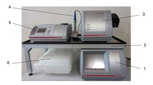
Fig. 22 - 16 Lovis 2000 ME + DMA M + pH ME + Abbemat + Xsample 122/520 - Placing master instruments and modules
