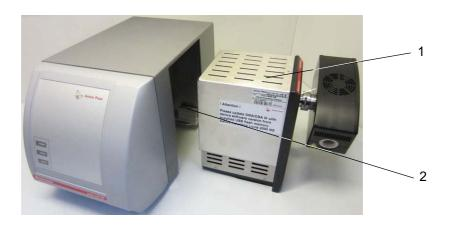
Fig. 6 - 4 Inserting the Lovis 2000 ME Microviscometer Module
