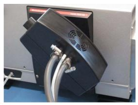
Fig. 6 - 12 Standard cooling hoses and dry air supply on the Lovis capillary block
