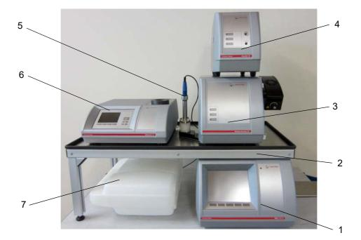
Fig. 22 - 20 Lovis 2000 ME + DMA M + HazeQC ME + pH ME (Bev.) + Abbemat + Xsample 122/520 - Placing master instruments and modules
