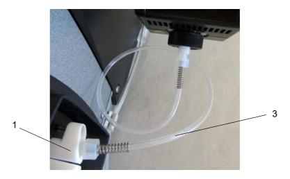
Fig. 21 - 2 Connecting the hose between DMA M and Lovis
