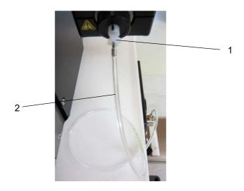
Fig. 18 - 10 Mounting the hose between Xsample needle and Lovis
