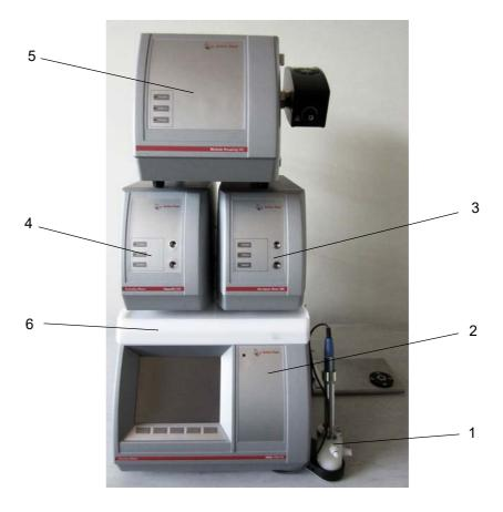
Fig. 20 - 2 Placing master instrument and modules - vertical setup
