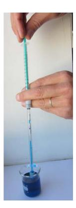
Fig. 9 - 4 Drawing in sample from a vessel
