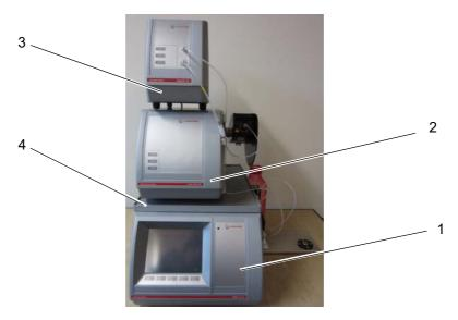
Fig. 20 - 25 Placing master instrument, Lovis 2000 ME and HazeQC ME
