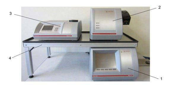
Fig. 22 - 23 Lovis 2000 ME + DMA M + Abbemat + Xsample 352/452 - Placing master instrument and modules
