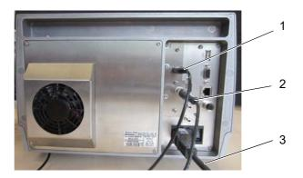
Fig. 21 - 8 Connecting the cables
